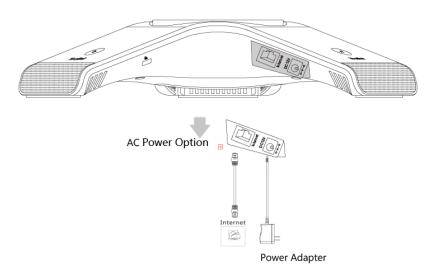
Note The IP phone should be used with Yealink original power adapter (12V/1A) only.
