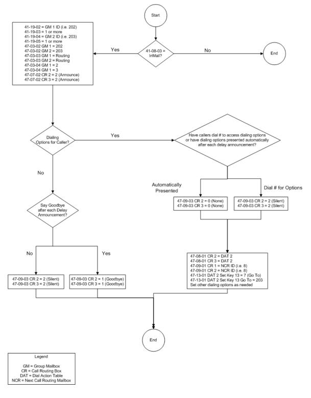
Figure 3-1 ACD Delay Announcement Flowchart
