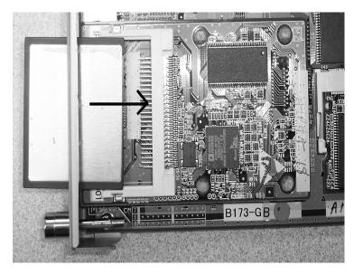
Figure 1-2 InMail Daughter Board with CompactFlash Card Assembly Installed
