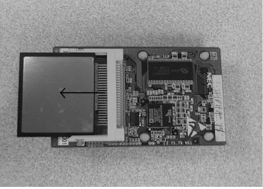
Figure 4-4 Removing the CompactFlash Card from the Blade
