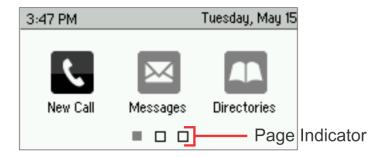
To change the displayed page, press the down or up arrow key. To change the highlighted entry, press the right or left arrow key. Press **Select** to access the desired menu.
